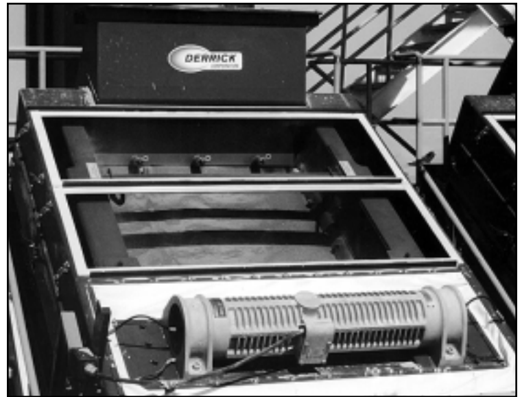
Derrick A56-168D-4M producing -35 mesh phosphate product.
